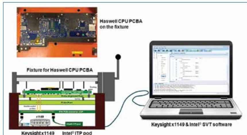
**FIGURE 5.** Small footprint solution comprising a Haswell CPU PCBA fixture, Intel ITP pod, x1149 boundary scan analyzer and software on a Windows 7 PC.
