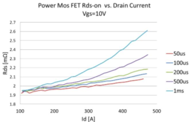
Figure 3: Pulse width dependency of  $R_{\text{ds,on}}$  measurement
