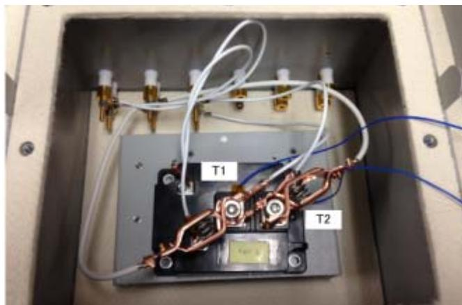
Figure 8: FUJI Electronics IGBT 1MBI800U4B-12 1- Pack module
