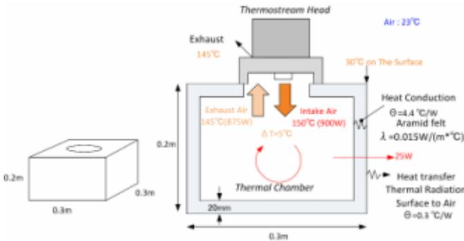
Figure 6: Thermal enclosure heat transfer block diagram
