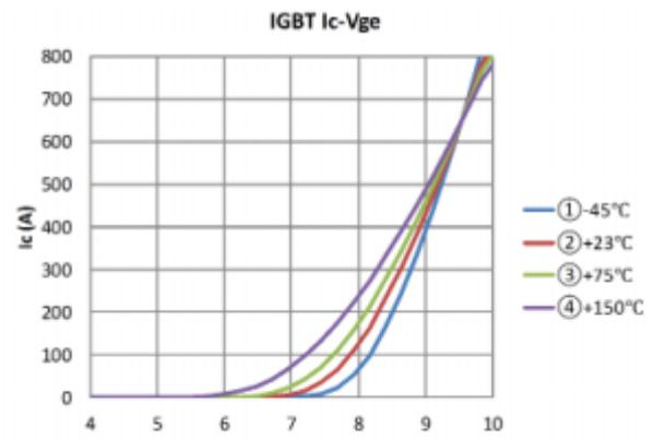
Figure 11: IGBT Ic-Vge characteristics at different Thermostream\* temperatures
