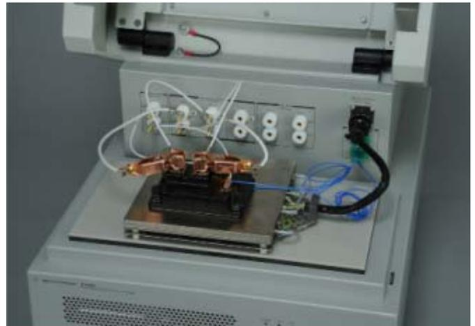
Figure 4: Thermal plate in B1506A test fixture
