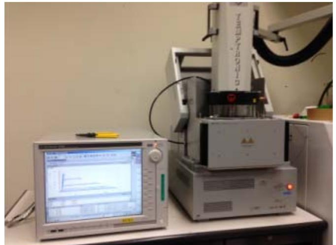
Figure 5: B1506A Test Fixture Thermal Enclosure for Thermostream\*
