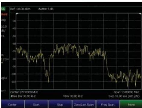
In traditional SA mode, it is hard to find the interfering signal buried inside the downlink carrier
