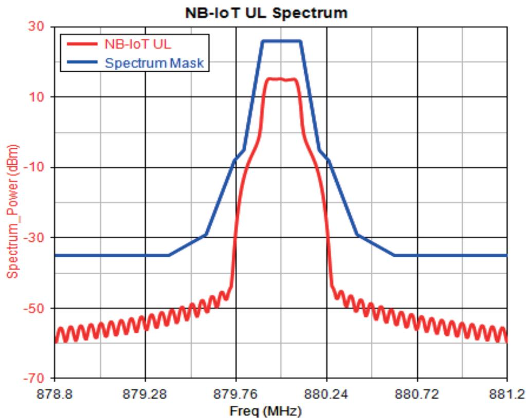
Figure 1. Example of a NB-IoT UL transmitting signal with 15 kHz subcarrier spacing, NPUSCH format; 1,12 subcarriers and a spectrum mask (blue).
