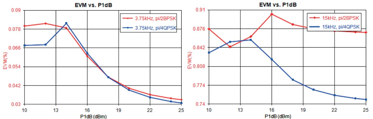
Figure 7. EVM vs. P1dB for a backed off PA with a single tone transmission with 3.75 kHz (left) and 15 kHz (right) subcarriers. We used a 200 kHz bandwidth digital filter. The PA input power was 20 dBm and gain was set to 0 dB intentionally for the simulation.
