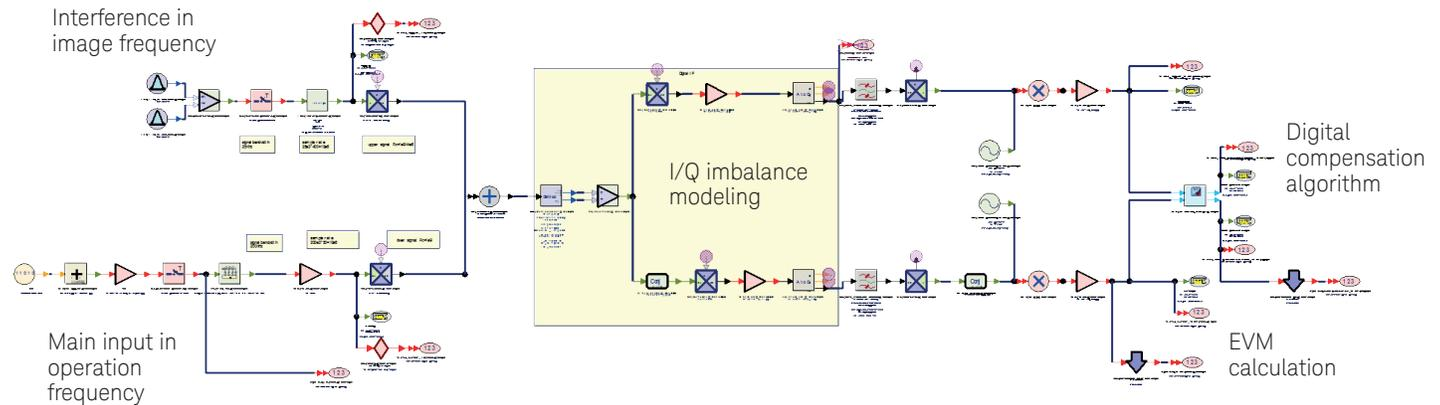
Figure 5. Simulation setup for Low-IF receiver I/Q imbalance compensation.
