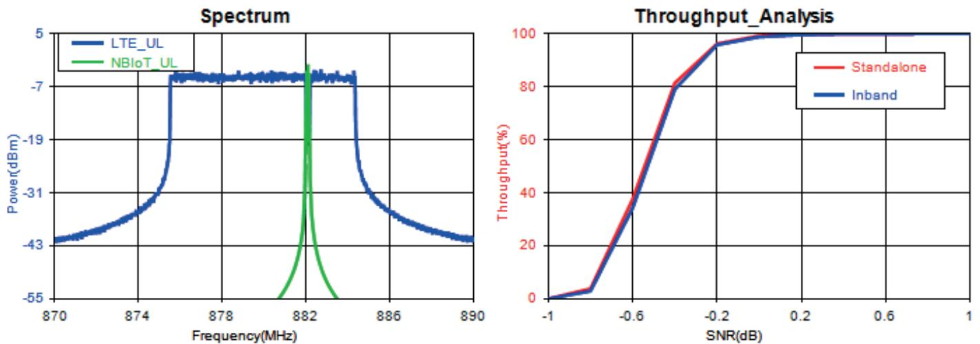
Figure 2. An in-band operation uplink coexistence analysis with a victim LTE (10MHz) and an aggressor NB-IoT device. Two spectrum traces (left) intentionally separated and overlapped in the same plot. Total 1000 LTE sub frames transmitted to throughput analysis.
