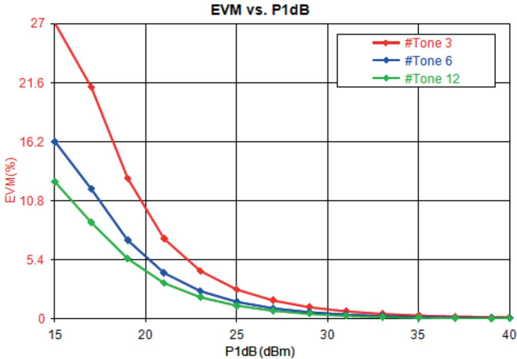
Figure 8. EVM vs. P1dB for a backed off PA with a multi-tone transmission with 15 kHz subcarriers. The digital filter is bypassed. Input power of PA was 20 dBm and gain was set to 0 dB intentionally for the simulation.
