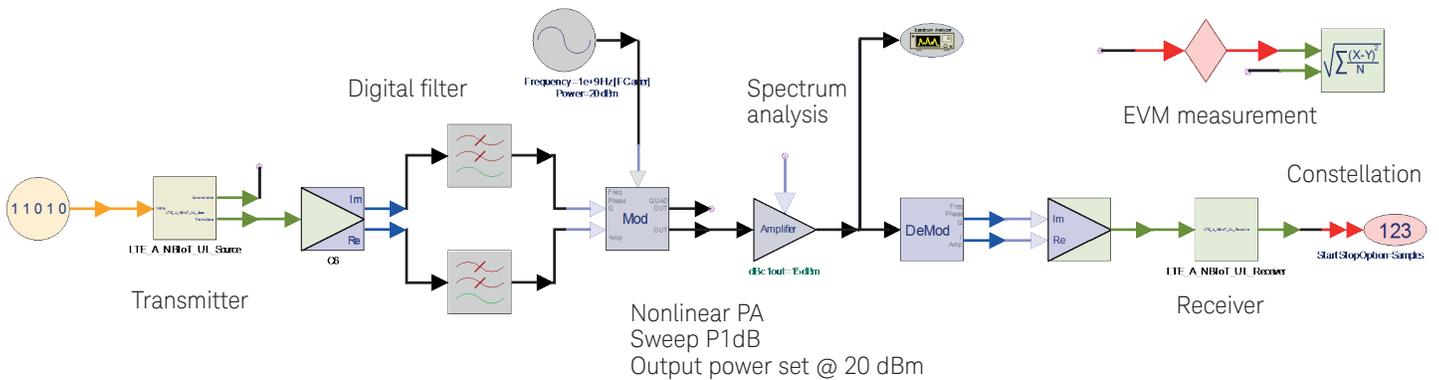
Figure 6. Simulation setup for the NB-IoT Uplink.
