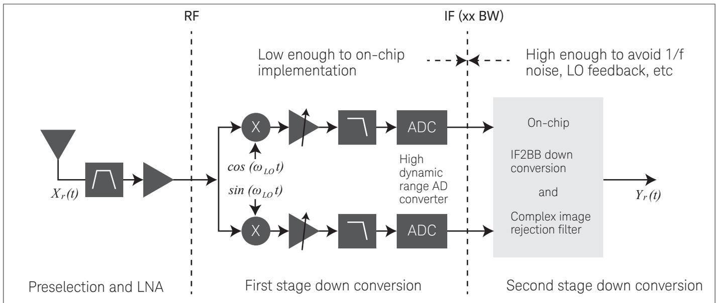
Figure 4. Low-IF receiver architecture.
