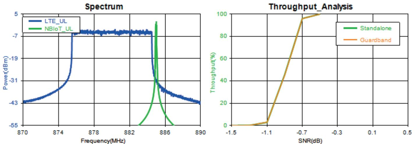
Figure 3. A guard-band operation uplink coexistence analysis with a victim LTE (10MHz) and an aggressor NB-IoT device. Two spectrum traces (left) intentionally separated and overlapped in the same plot. A throughput analysis (right) of a total of 1000 LTE transmitted subframes.
