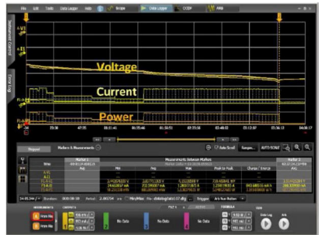
Figure 4. Battery run down test result
