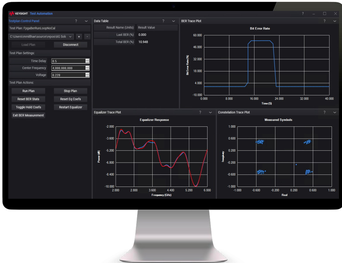
Figure 6. Real-time data displays built from dockable panels in the PathWave Graphical Editor
