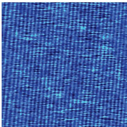
Figure 1. High resolution AFM topography image of  $C_{36}$  alkanes on HOPG substrate, captured at 100 lines/s. Image scan size is 150 nm × 150 nm.
