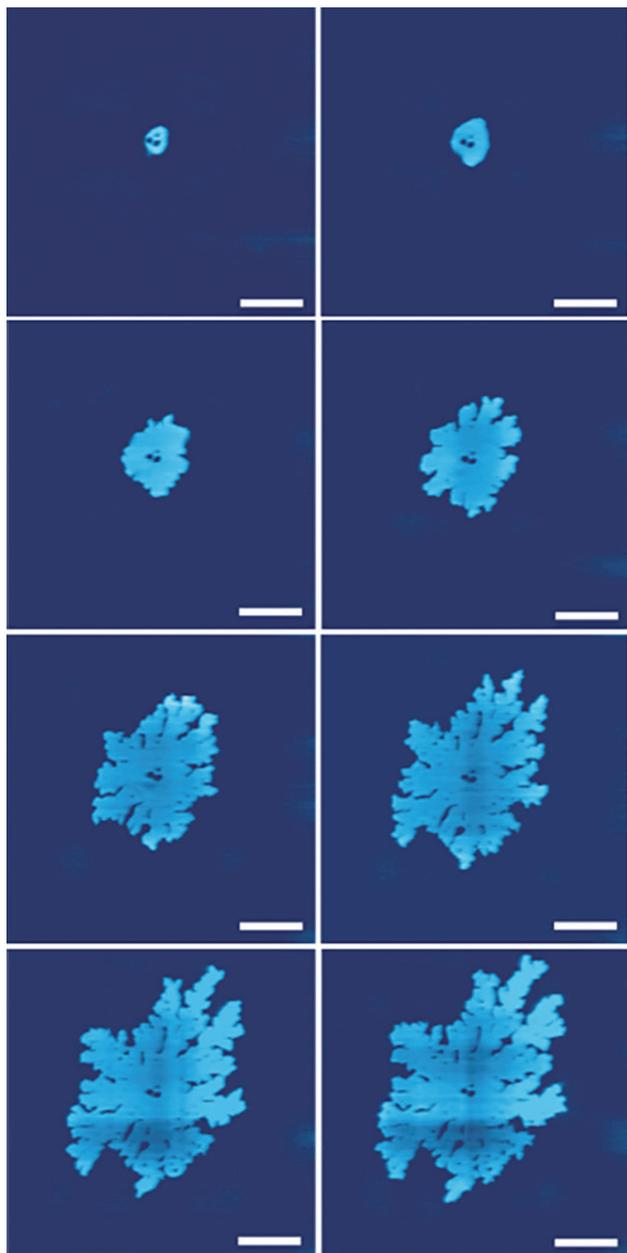
Figure 3. Every fourth AFM images obtained through AAC QuickScan mode illustrating the progressive growth of ice crystal formation, starting from a small nucleus into a structure with many branches. AFM imaging was performed at 0.4 frame/s. Scale bar is 1  $\mu\text{m}$ .
