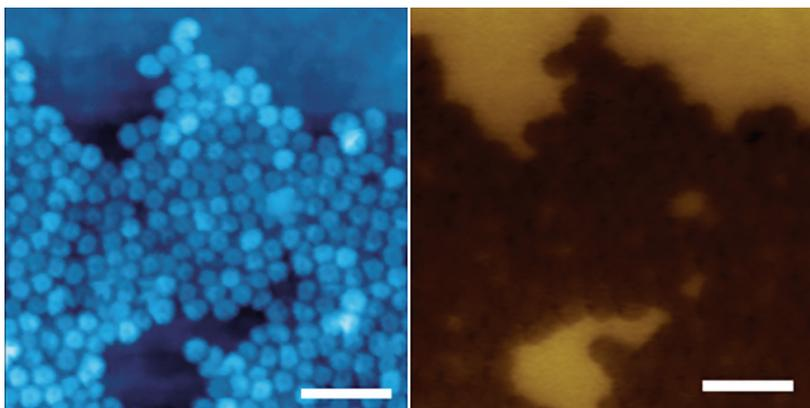
Figure 4. Topography (left) and surface potential (right) images of  $\text{F}_{14}\text{H}_{20}$  fluoroalkane self-assembly on Si substrate, obtained at 60 lines/s. Scale bar is 200 nm.
