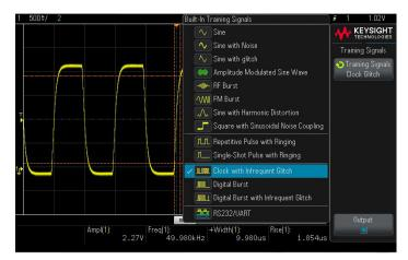
A large variety of training signals supply common test and analysis signals for users to gain expertise in oscilloscope usage and signal analysis.
