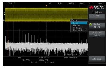
$\label{eq:multiple} \mbox{Multiple FFT window functions are supported to provide required signal analysis.}$
