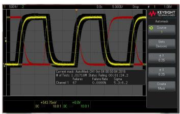
Mask testing can quickly validate signal quality and detect errors.
