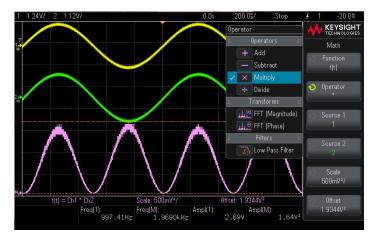
Easily calculate the resulting waveform when adding two waveforms by using waveform math.
