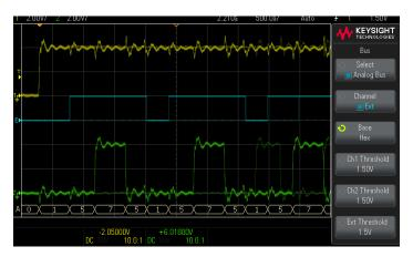
Channel 1, 2 and external trigger can be combined to form a bus with hex or binary values displayed as the bus along the bottom of the display.
