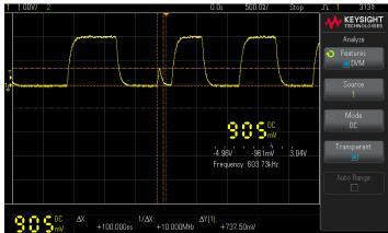
The DVM makes accurate RMS measurements when the signal frequency is between 20 Hz and 100 kHz.
