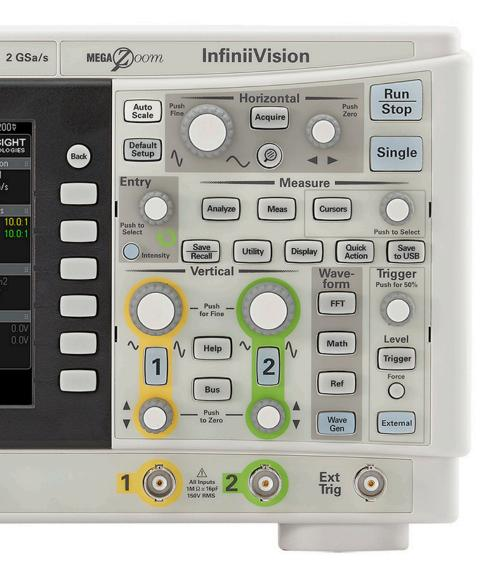
Custom measurements are easy with "Cursors." Measure any value or the difference using four powerful cursors.
