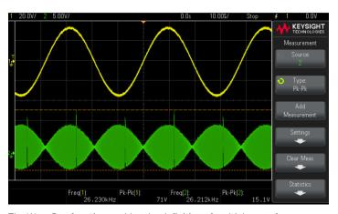
The WaveGen function enables the definition of multiple waveforms including amplitude modulated signals.
