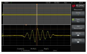
Zoom in to see signal detail, and use the cursors to easily make exact measurement.
