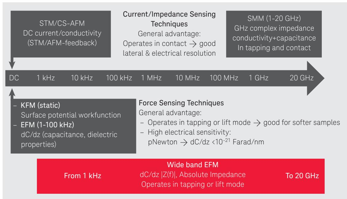
Figure 1. Electrical AFM techniques and their operating frequency range. SMM (scanning microwave microscopy); KFM (Kelvin force microscopy); EFM (electrostatic force microscopy); CS-AFM (current-sensing AFM).
