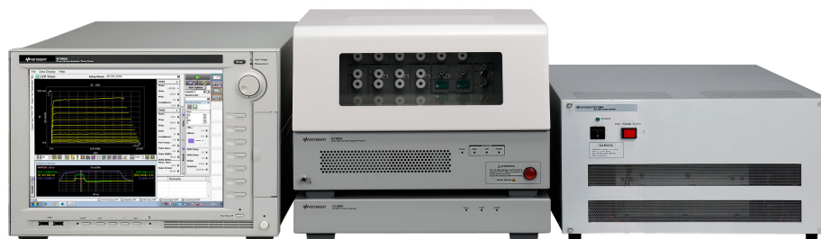
Figure 1.15. The B1505A power device analyzer/curve tracer with its ultra-high current and ultra-high voltage modules.
