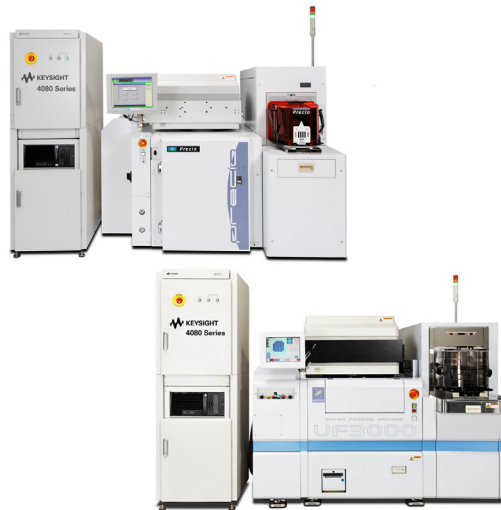
Figure 1.3. A production parametric tester is designed to optimize throughput
