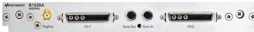
Figure 5.24. The B1500A's WGFMU module can output 10 V peak-to-peak and has a minimum pulse width of 50 ns.
