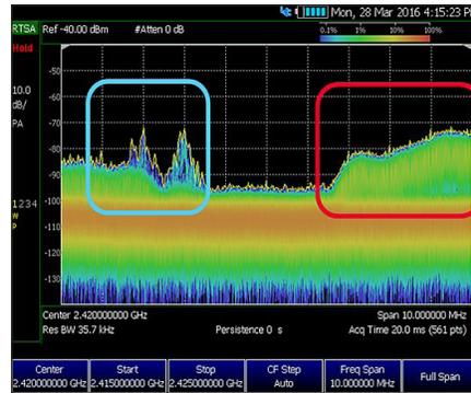
Figure 4. With RTSA features, user can identify multiple types of signals in the same frequency band. The Bluetooth® signal is highlighted in blue while the wireless LAN signal is in red.
