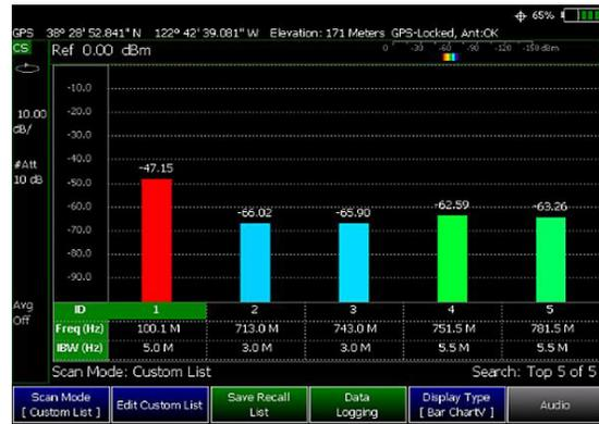
Figure 2. This screenshot shows the wireless network channels present in an active area. FieldFox scans up to 20 channels simultaneously at any given frequency and bandwidth.
