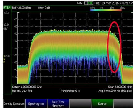
Figure 5. RTSA offers a measurement display called density display, providing signal hitting capabilities at specified frequency span. This feature makes it easier to identify two different signals that have power level fluctuations with distinct statistic natures. This screenshot illustrates how RTSA can clearly see the "threat" instantly.
