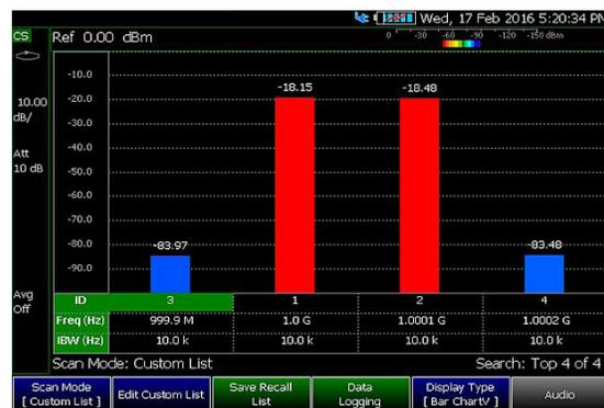
Figure 3. Targeted signal strengths and new intermodulation signals.
