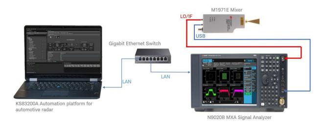
The E8740A-010 solution provides cost-effective testing for automotive radar RF, from 3 Hz to 26.5 GHz and 60 GHz to 90 GHz including RF analysis and access to test standards with KS8320A.
