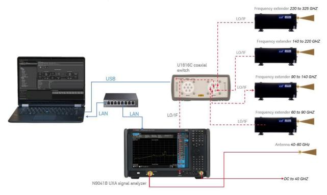
The E8740A-090 solution provides all of the hardware components for you to analyze signals from 0 - 330 GHz for emission testing. Tests include; operating frequency range, mean power, peak power, unwanted emissions in the out-of-band domain as well as unwanted emissions in the spurious domain for both transmitter and receiver conformance.
