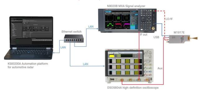
The E8740A-040 covers frequencies 3 Hz to 26.5 GHz as well as higher banded 60-90 GHz and with 2.5 GHz bandwidth verify the accurate transmission of radar signals for both 24 GHz and 77/79 GHz. Use it for RF test with an FFT and FMCW signal quality including harmonic, spurious, and spectrum emissions, phase noise, analog/digital I/Q input, modulation quality, linearity, as well as other measurements.
