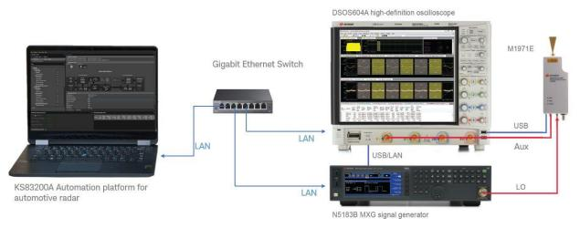
The E8740A-020 solution provides a testing configuration for automotive radar signal quality verification. Expand to simultaneous two channel analysis with two M1971E mixers set at the same frequency. Make RF power, frequency stability, modulation quality, RF and FMCW signal quality measurements. The E8740A-020 will provide in-band measurements for your radar transmitter systems.
