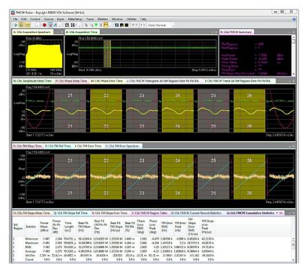
View spectrum and time domain results on multichirp FM signals. In the image pictured here highlighting six selected FM regions (number 21 through 26) in synchronized time domain traces. The FMCW cumulative statistic table below provides accumulated results over all detected regions.
