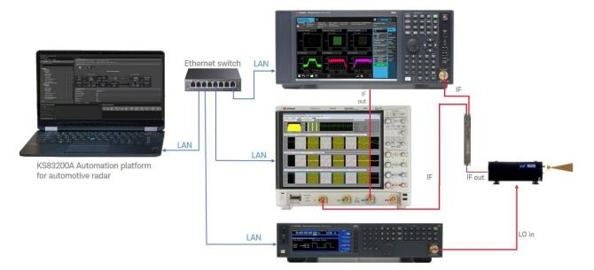
The E8740A-050 solution provides the frequency and bandwidth to accurately test both short range and longrange radar. Capture, analyze and test RF signals with an FFT or use it for FMCW signal quality including spectrum emissions, phase noise, modulation quality, linearity, and more measurements. If you need a wider frequency sweep or wider bandwidth, please consider our most advanced signal analysis option with the E8740A-060.
