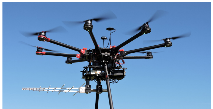
Antenna pattern measurements using UAV
