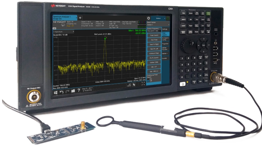
Near-field probe and CXA signal analyzer test the emission of PC LAN port during design cycle before full compliance testing.
