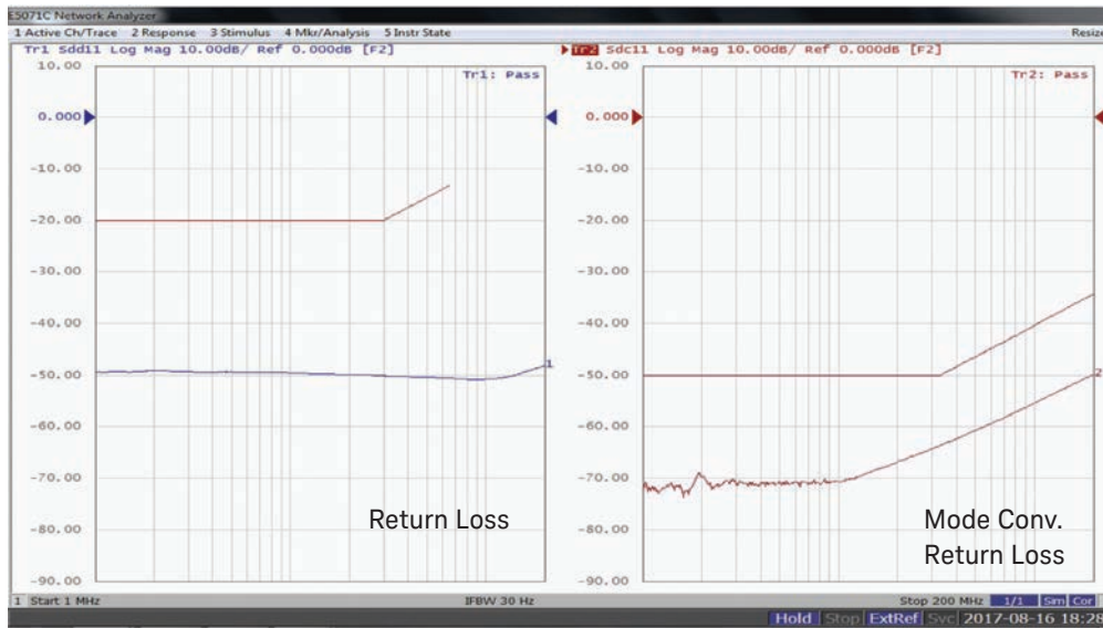
Figure 5. E6964A MDI S-parameter typical display.
