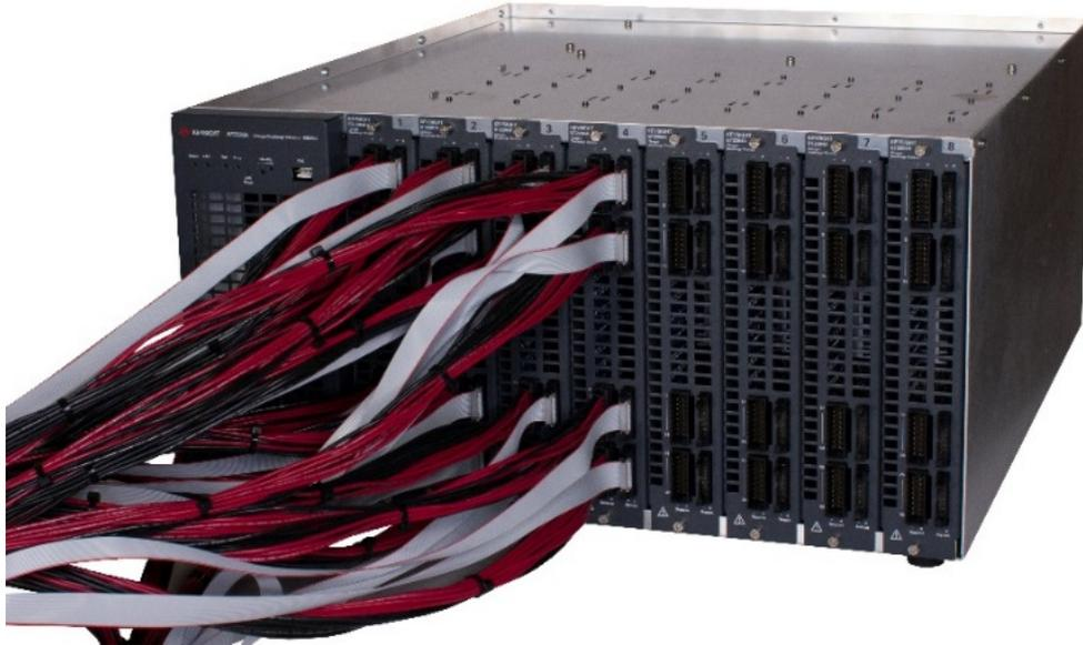
Figure 2 - Paralleled wiring connections create configurable charge-discharge channels up to 200 A.
