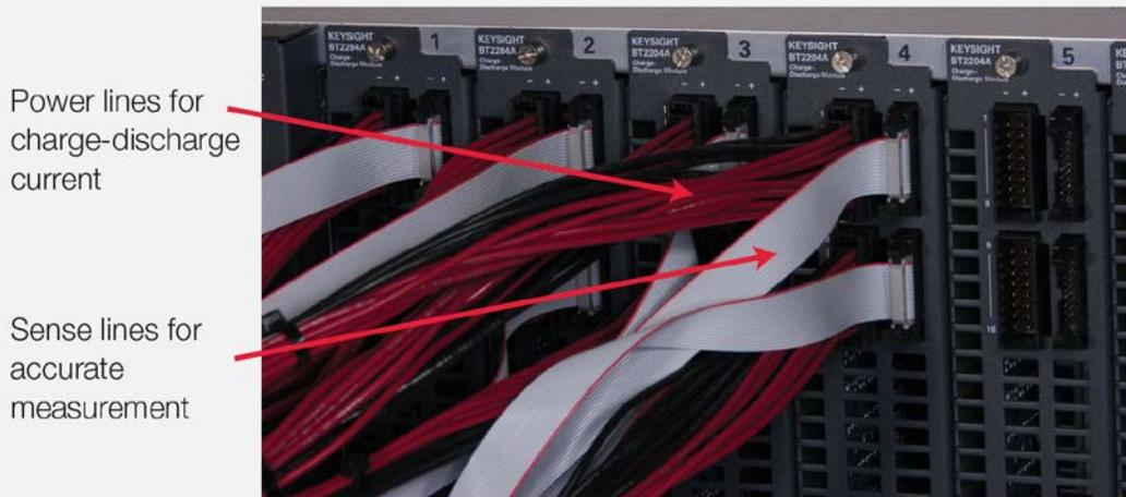
Figure 3 - 4-wire connections (power and sense) to cells enable accurate measurements even with long cables to your fixture
