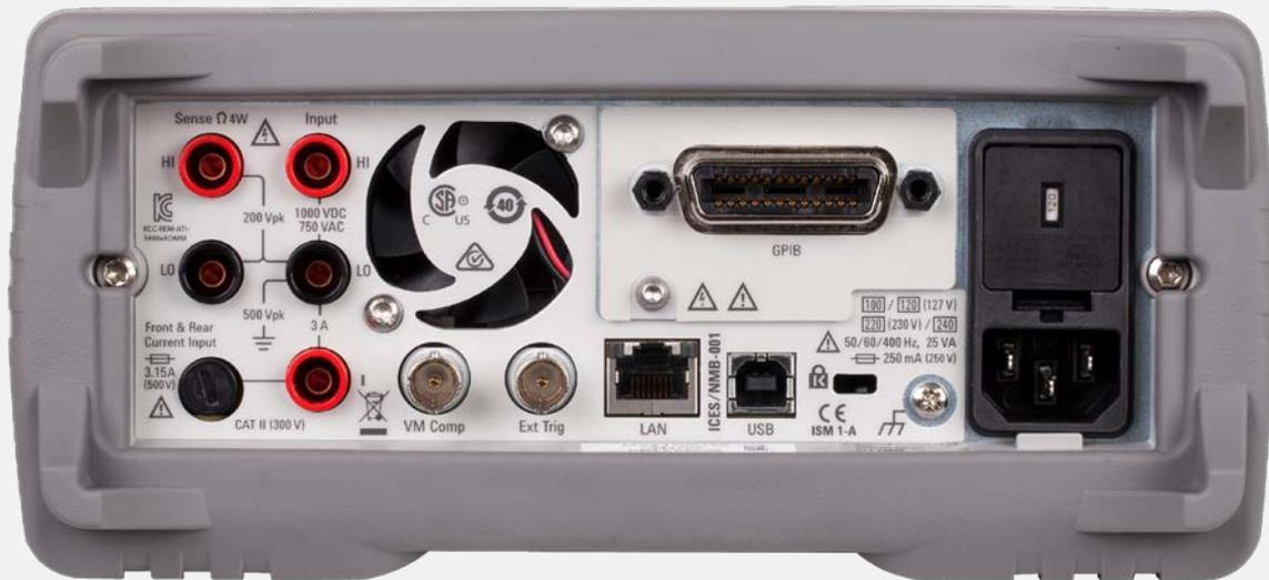
Figure 1: Example of the 34470A digital multimeter's rear panel showing warnings on the maximum voltage input and maximum current input
