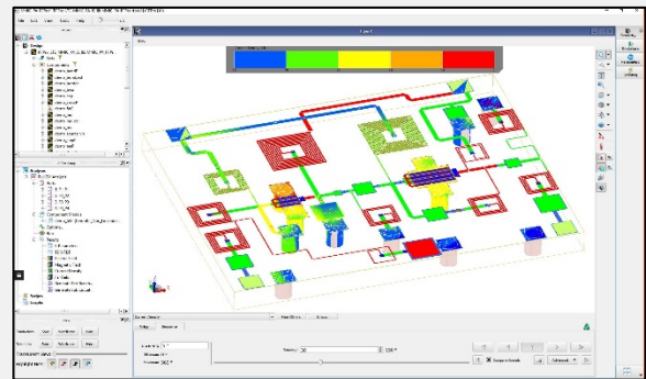
Predictive EM expert settings makes EM-circuit co-simulation of this MMIC as easy as circuit simulation
