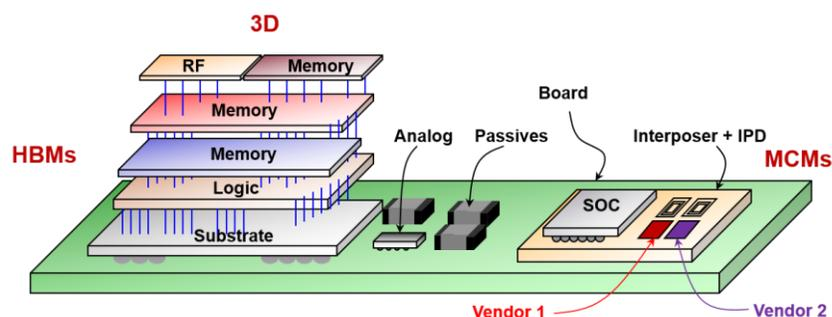
Figure 1: PCBA with Advanced Packaging and Multi-Chip Modules
