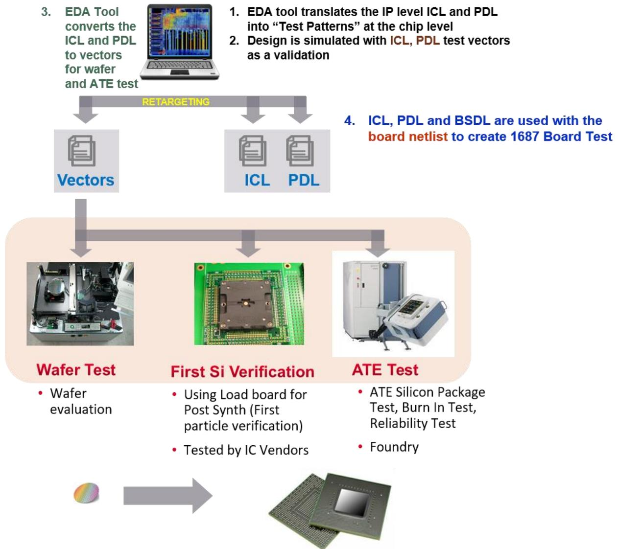
Figure 5: IEEE 1687 in Silicon Flow
