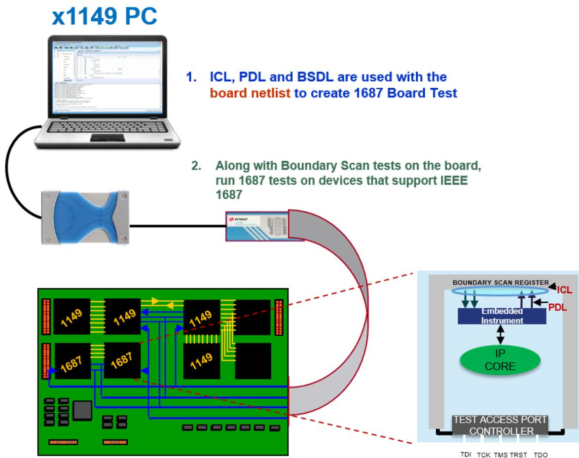
Figure 6: IEEE 1687 in Board Test Flow
