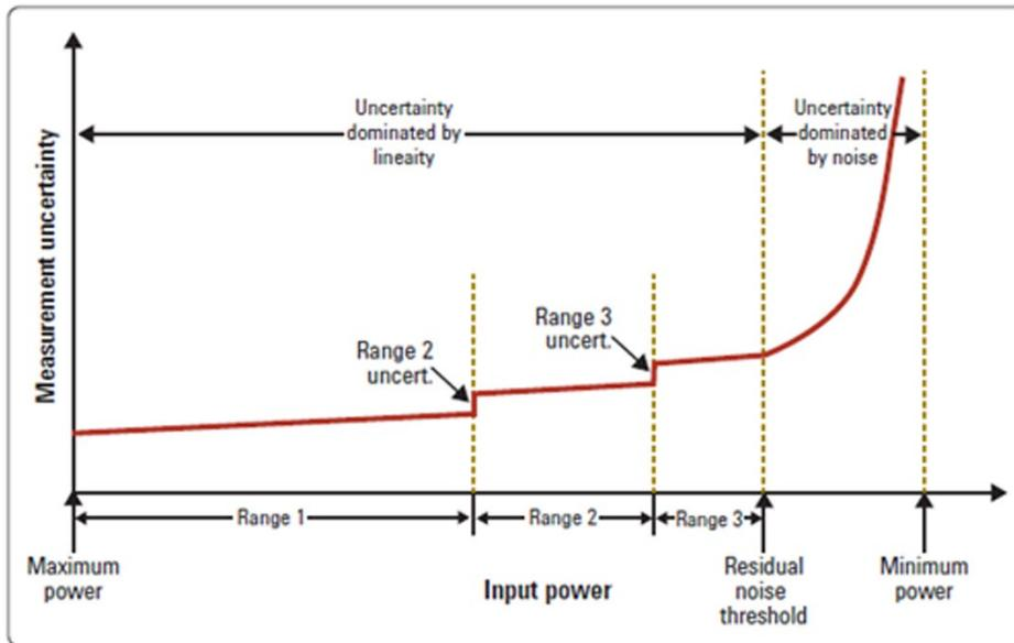
Figure 5. Measured uncertainty vs. input power relationship
