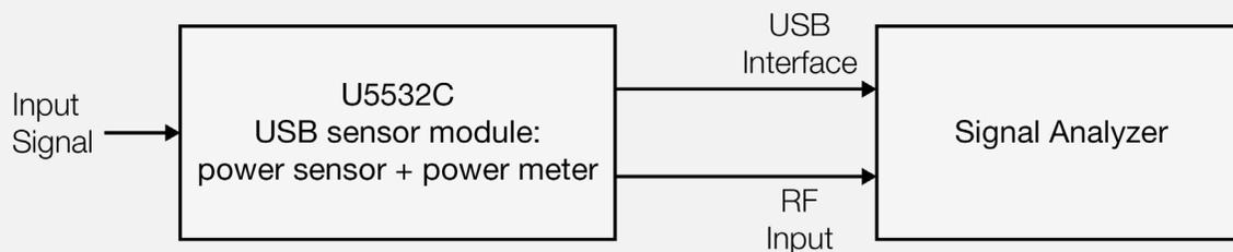
Figure 1. Primary configuration for the N5531X measuring receiver
