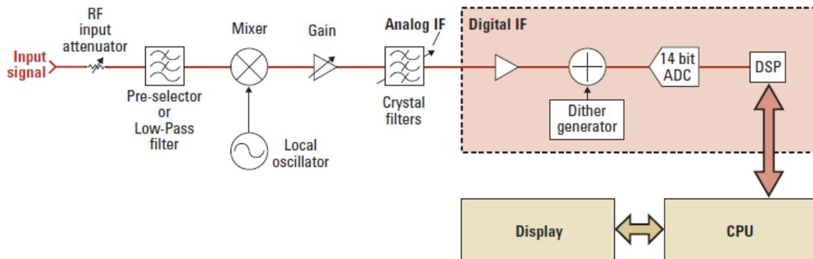
Figure 4. Simplified block diagram of the PXA signal analyzer
