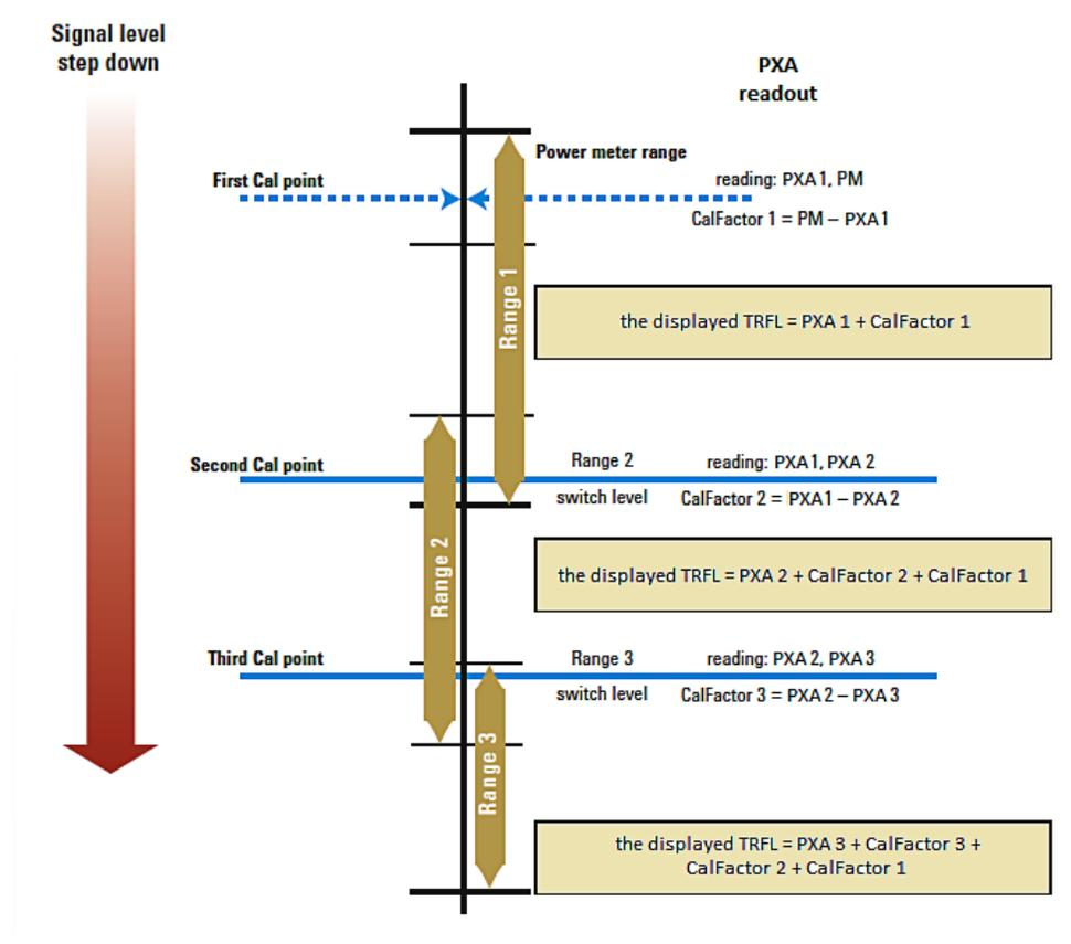
Figure 3. TRFL ranging calibration
