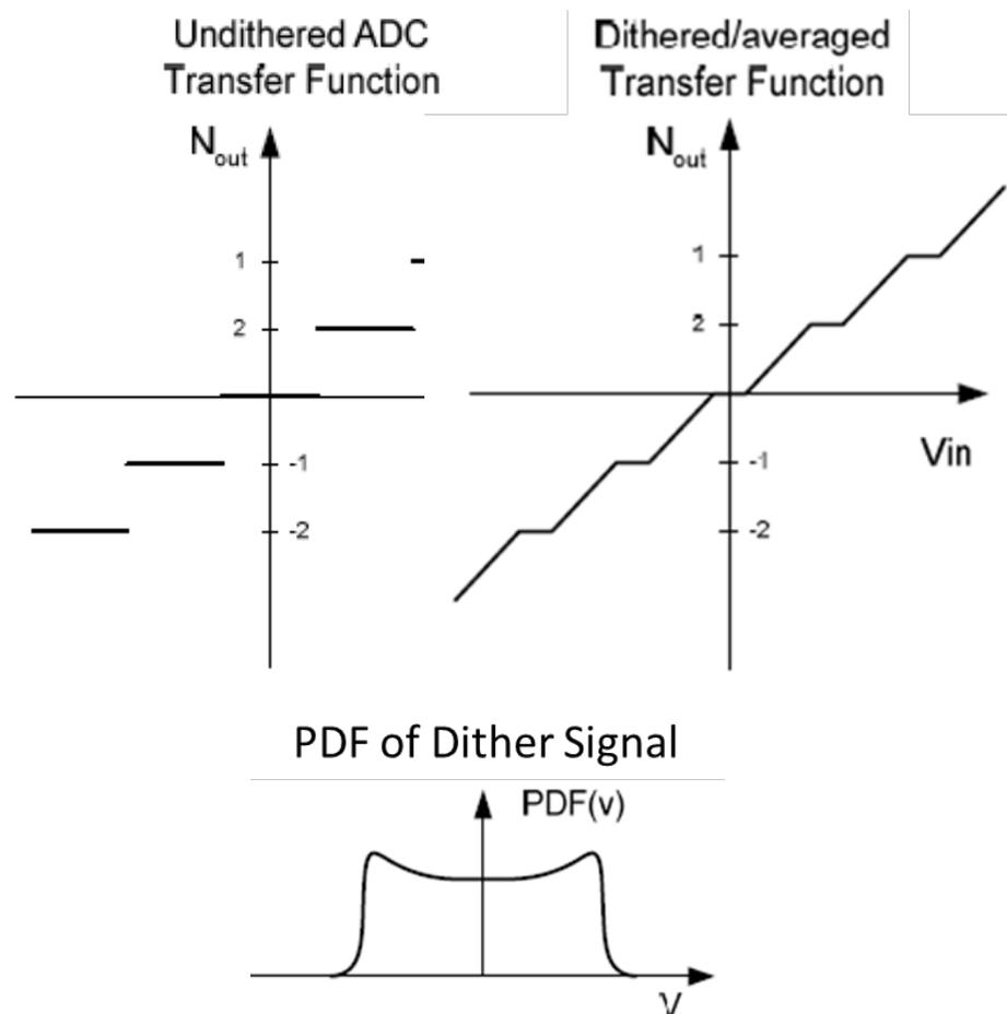
Figure 6. ADC linearity
