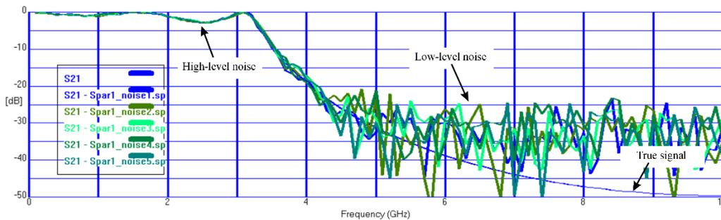
Figure 12: Simulation of the effect of noise floor and trace noise superimposed to ideal data on a Low pass filter measurement
