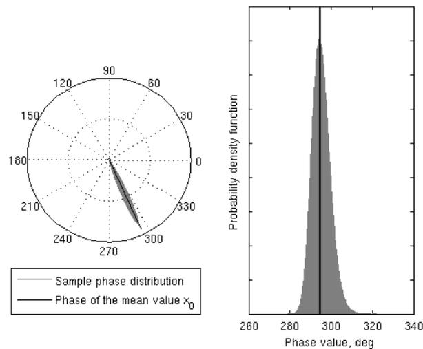
Figure 3: Phase histogram of repeated complex data measurements.
