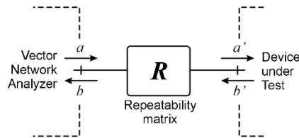
Figure 14: Connector and cable repeatability model.
