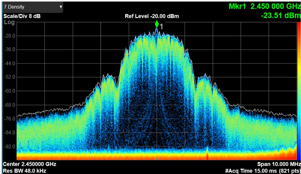
Figure 2: A ZigBee signal is about 3 MHz wide
