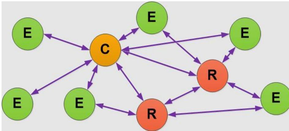
Figure 1: ZigBee can form a mesh network of mixed node types to forward messages
