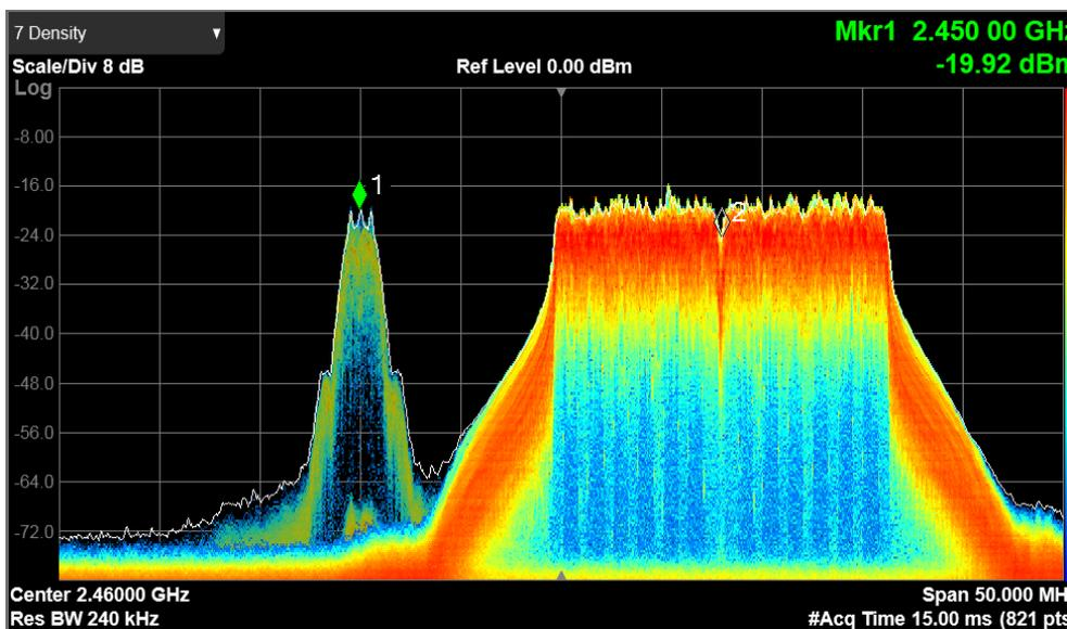
Figure 3: A ZigBee signal (left) is much narrower than a Wi-Fi signal (right)
