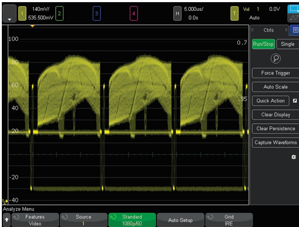
Figure 6. Triggering on 1080p HDTV.
