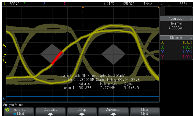
Figure 4. MIL-STD 1553 eye-diagram mask test.
