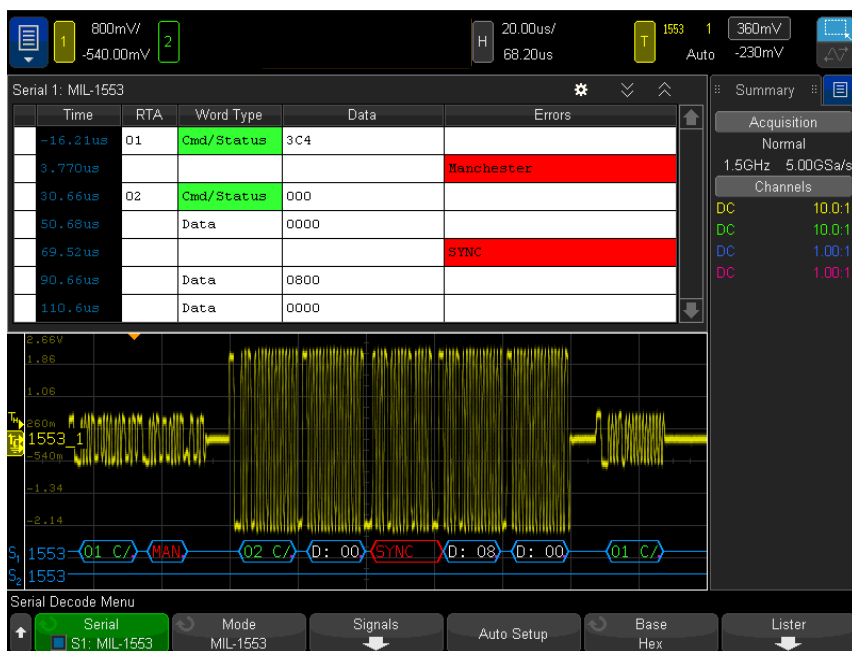
Figure 2. MIL-STD 1553 decode on an InfiniiVision X-Series oscilloscope.
