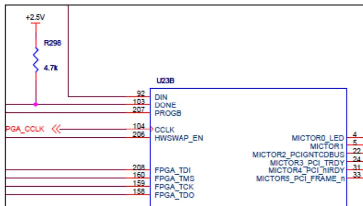
Figure 1-6: Sample of none pull up in the circuit
