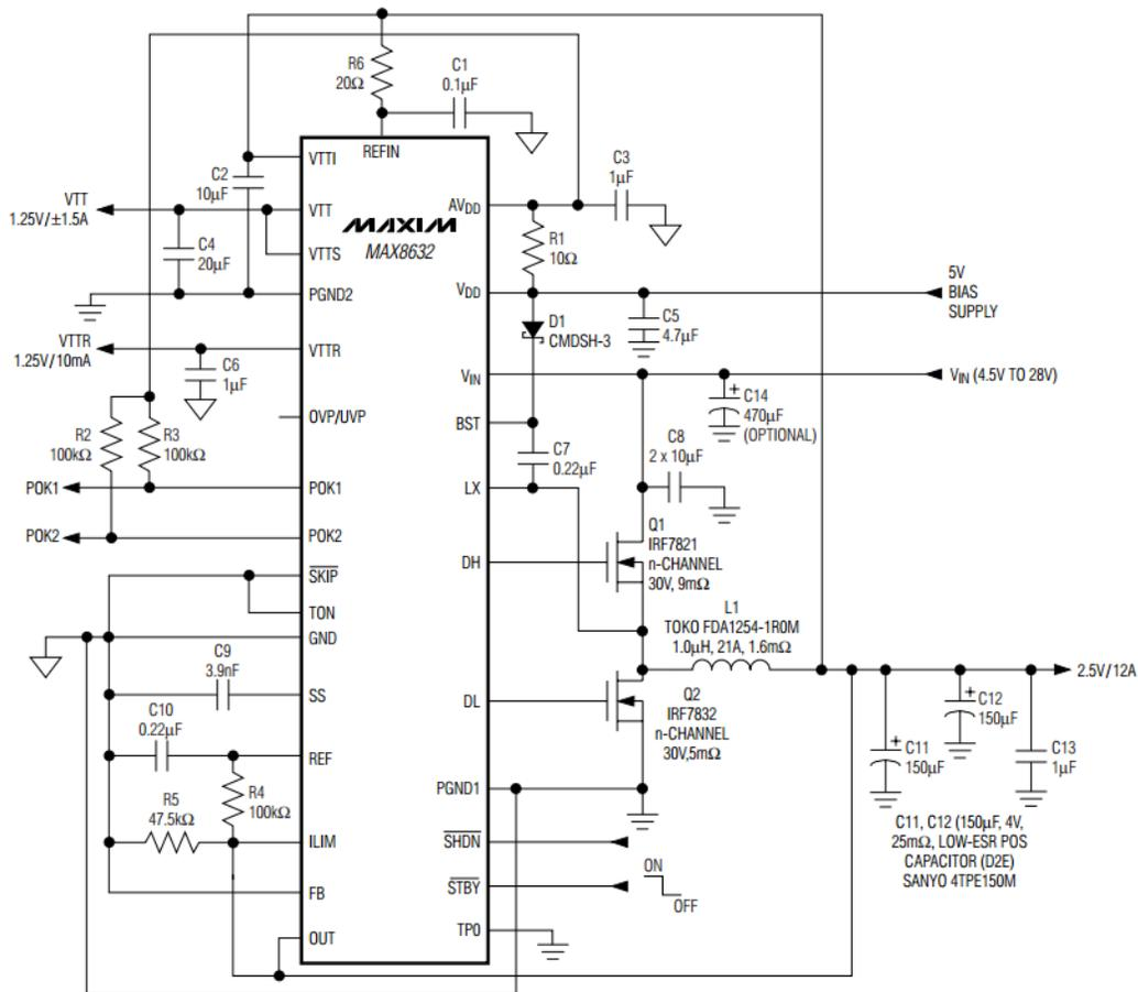
**Figure 1-3: Typical PWM Circuit**
