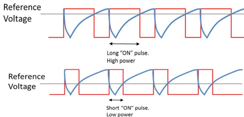
**Figure 1-2: MOSFET ON/OFF Wave**
