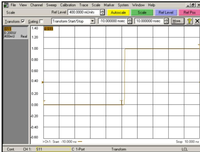
If the time-domain reflectometer (TDR) is showing a unity reflection step as specified above, the sensor is considered to have been overloaded with too much power.
