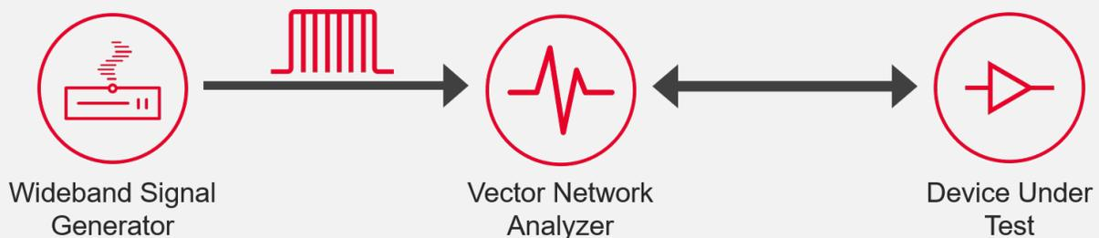
Figure 3: External wideband source provides test signal to DUT through VNA
