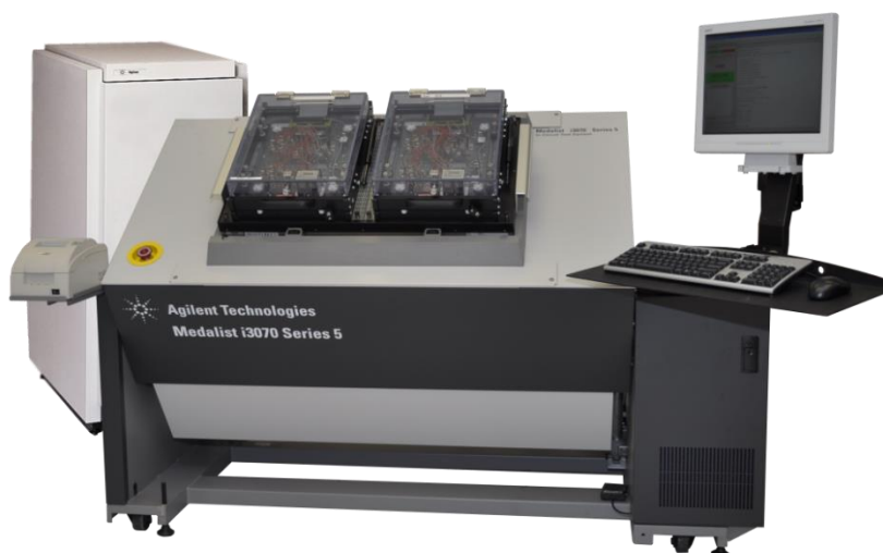
Figure 1. i3070 Series 5 with consists of an ASRU revision N card, Control XTPA card, and iSystem card
