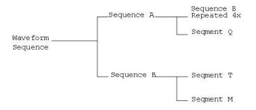
The following procedure describes how to create two waveform segments, then name and store them in ARB memory. After you name and store the two waveform segments in ARB memory, you can use them to build a waveform sequence, as described on page 119.
