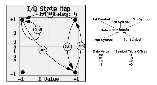
When applied to the user-defined default 4QAM I/Q map, starting from the 1st symbol (data 00), the differential encoding transitions for the data stream (in 2-bit symbols) 0011100001 appear in the previous illustration.
