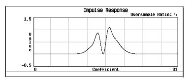
The graphic display can provide a useful troubleshooting tool (in this case, it indicates that a coefficient value is set incorrectly, resulting in an improper Gaussian response).
