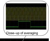
The ALC samples the waveform when the marker signal goes high, and uses the average of the sampled waveform to set the ALC circuitry.
