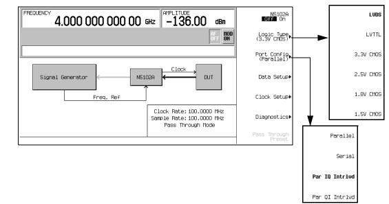
Figure 12-16 Logic and Port Configuration Softkey Menus
