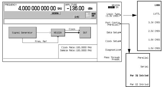
1. Refer to Figure 12-10. Press the Logic Type softkey.
