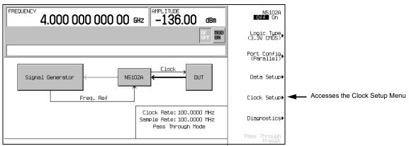
From this softkey menu, set all of the clock parameters that synchronize the data between the N5102A module and the device. From this menu, the clock signal phase can be changed so the clock occurs during the valid portion of the data. Figure 12-18 shows the clock setup menu.
