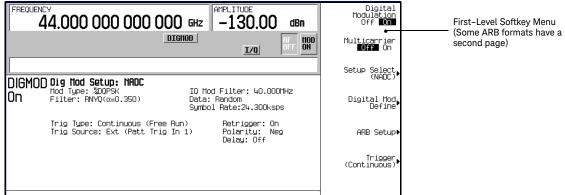
At this point, a default file header has been created, with default (unspecified) settings that do not reflect the current signal generator settings for the active modulation. To save the settings for the active modulation, you must modify the default settings before you save the header information with the waveform file (see "Modifying Header Information in a Modulation Format" on page 107).
