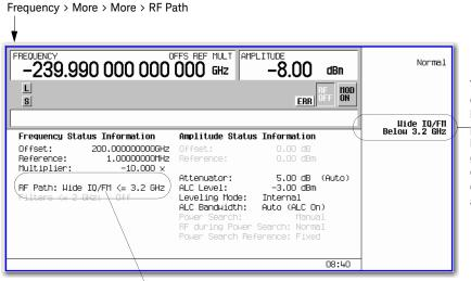
This softkey selects the downconverted RF path below 3.2 GHz. When this path is active, the low band frequencies are generated by a downconverter. This enables very wide I/Q and FM performance.
