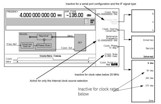
The top graphic on the display shows the current clock source that provides the output clock signal at the Clock Out and Device Interface connectors. The graphic changes to reflect the clock source selection discussed later in this procedure. The bottom graphic shows the clock position relative to the data. The displayed clock signal will change to reflect the following:
