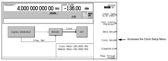
From this softkey menu, set all of the clock parameters that synchronize the clocks between the N5102A module and the PSG. You can also change the clock signal phase so the clock occurs during the valid portion of the data. Figure 12-14 shows the clock setup menu.
