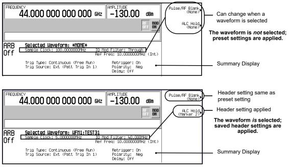
Basic Digital Operation Using the Dual ARB Waveform Player
