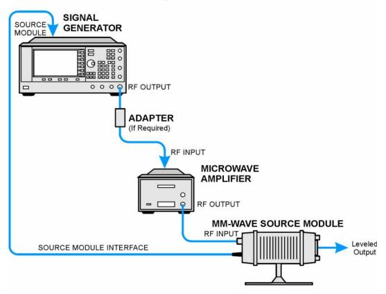
Figure 12-22 Setup for E8267D PSG and E8257D PSG with Option 1EA, 1EU, or 521
