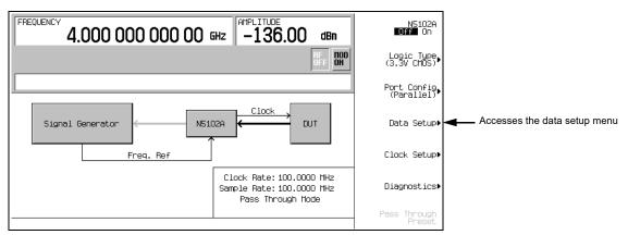
This softkey menu accesses the various parameters that govern the data received by the PSG. The status area of the display shows the number of data lines used for both I and Q along with the clock position relative to the data. Figure 12-20 shows the data setup menu structure.
