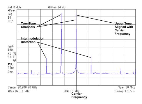
Two-Tone Waveform Generator Creating, Viewing, and Modifying Two-Tone Waveforms Keysight Technologies E8257D/67D & E8663D PSG Signal Generators
