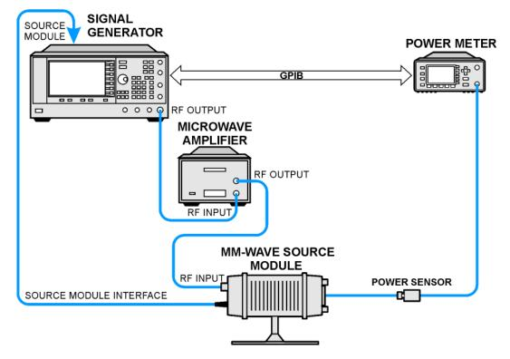
Figure 4-6 User Flatness with mm–Wave Source Module for Signal Generators with Options 1EA, 1EU, or 521
