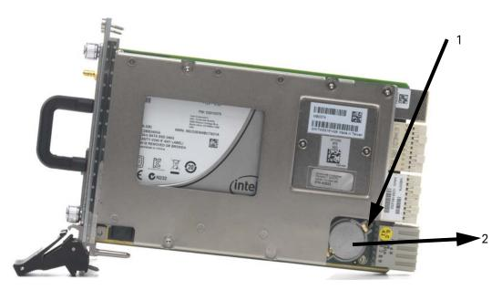
**Figure 14** Replacing the Battery
