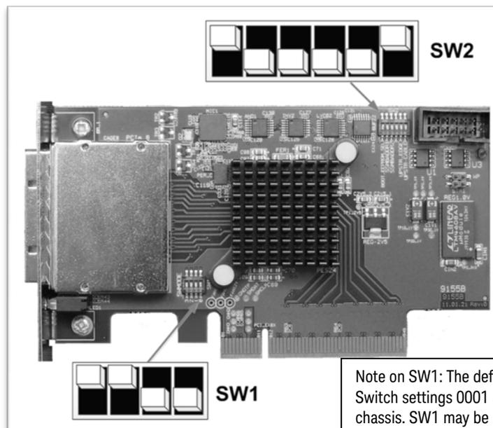
Note on SW1: The default setting (1100) is shown in the graphic. Switch settings 0001 are also acceptable for use with Keysight chassis. SW1 may be removed on future versions of the M9048A.
