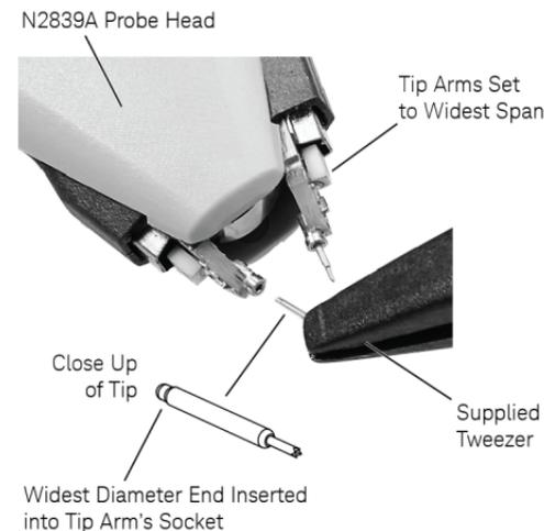
**Figure 4** Inserting a tip
