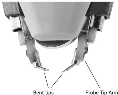
**Figure 3** Example of a damaged tip
