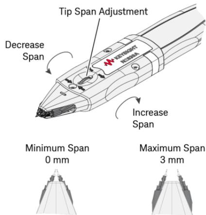
Figure 1 Adjusting the tip span
