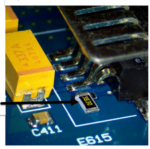
383 ohm 0699-1429 **5.** Add a 1/2 inch 32 gauge wire. Refer to Figure A-4.
