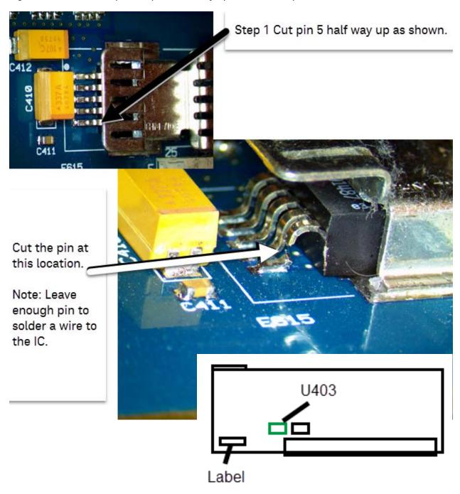
3. Clean pad and remove cut off portion of U403-pin 5 from the pad. Refer to Figure A-2.
