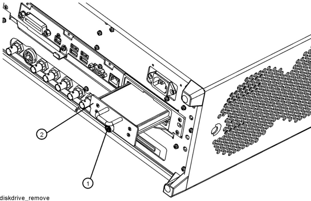
3. Replace the disk drive carrier assembly (2) into the instrument and tighten the screw (1) to 9 inch-pounds.
