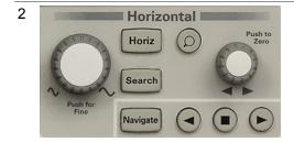
Configure the horizontal axis and navigate through the waveform.
