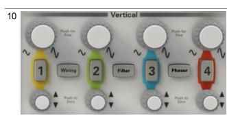
Press [1], [2], [3], or [4] to configure and display the voltage, current, and power channels, along with the associated channel sidebars. Use the scale and offset knobs to quickly zoom in on critical information. Use the [Wiring] key to specify how your DUT is wired to your instrument and to adjust channel the channel skew. Use the [Filter] key to select a high-pass filter, low-pass filter, or no filter for each channel. Use the [Phasor] key to configure and display a phasor diagram.
