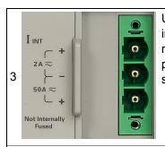
Use the three-pin connector (shown on channel 2) for either the internal 2-A (upper and middle pins) or 50-A (lower and middle pins) current shunts. Never connect to them simultaneously. On the front panel, press the channel key, then press **Current Input > Internal** to specify which shunt you are using.
