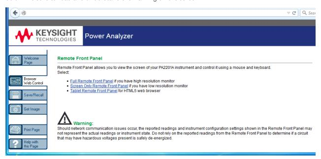
The Full Remote Front Panel option opens a window that contains an image of the front panel, including the knobs and keys. You can click on the keys, knobs, and display elements to run the instrument just as you would from the front panel. The PA2201A version is shown below; the PA2203A version also has channels 3 and 4 and the **[Filter]** and **[Phasor]** keys.
