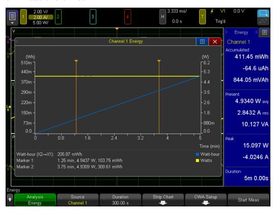
As mentioned above, you can press **Strip Chart > Strip Chart Type** to change the units. For example, the image below shows the strip chart with VA-Hour units. Note that the blue sidebar is not affected by this setting.
