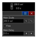
The horizontal scale knob works with both running and stopped acquisitions. When running, adjusting the horizontal scale knob changes the sample rate. When stopped, adjusting the horizontal scale knob lets you zoom into acquired data.
