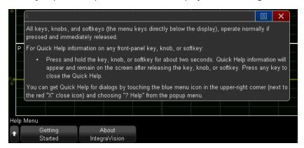
The **Getting Started** softkey contains additional helpful information about using the instrument; read through it to get up to speed quickly. The **About IntegraVision** softkey provides information about your instrument, including serial number, firmware revision, and where to download the latest firmware.
