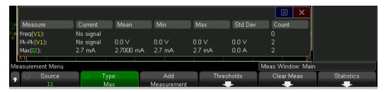
The source channel of the measurement is shown in parenthesis after the measurement name. For example: "Freq(V1)" indicates a frequency measurement on voltage channel 1. Statistics are based on the number of captured waveforms (count).
