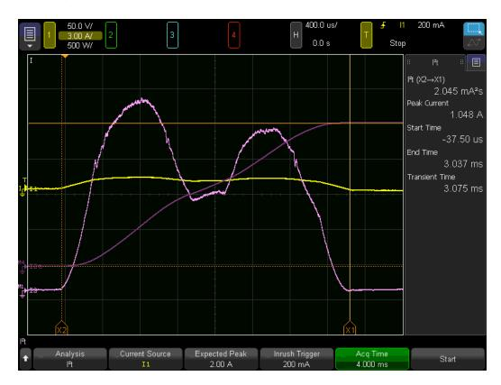
The bright horizontal yellow line is the current signal (I). It is yellow in this case because the Current Source is Channel 1. The bumpy, bright magenta line is a math function, the square of the current ( $I^2$ ). The rising purple line is the integral of the  $I^2$  signal over time ( $I^2$ t). The orange vertical and horizontal lines are the cursors delimiting the calculations shown in the sidebar.
