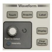
Use the knob above it to adjust the waveform intensity on a scale from 0 to 50.
