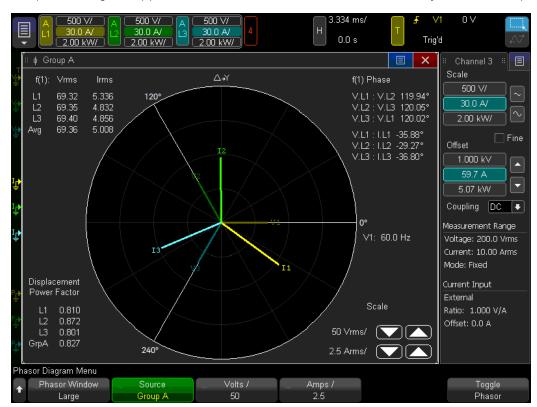
The horizontal axis of the phasor diagram (0 degrees) is defined as the phase of the voltage signal in the first channel in a wiring group, or the voltage signal of the selected channel if that channel is not part of a wiring group. All other phasors are shown in relationship to that.
