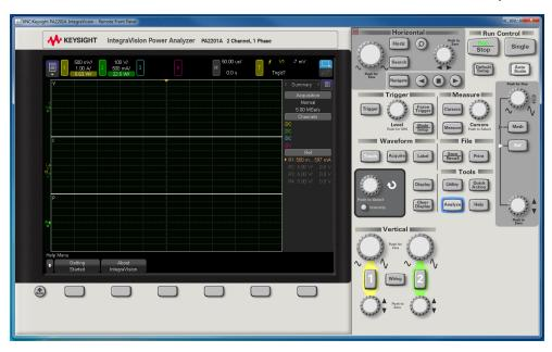
The Screen Only Remote Front Panel and Tablet Remote Front Panel also open in a separate window. You can operate the instrument just as you would using the touchscreen.
