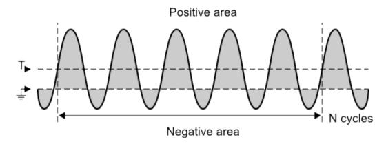
The Full Screen measurement interval variation measures the value on all displayed data points. The N Cycles measurement interval variation measures the value on a whole number of periods. If fewer than three edges are present, the measurement shows "No edges."
