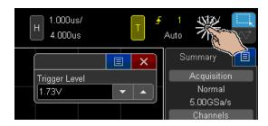
Touch "Auto" or "Trig'd" to quickly toggle the trigger mode.
