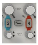
On the PA2201A or the PA2203A, you can press [Display] > Phasor, or you can use the blue menu symbol in the upper left corner of the display.
