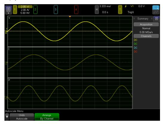
Press **Undo Autoscale** to return to the instrument's previous settings.
