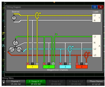
If, instead, the softkey for channel 1 had been set to 3P-4W-3M, then channels 1 through 3 would equate to lines 1 through 3, respectively, as shown below.
