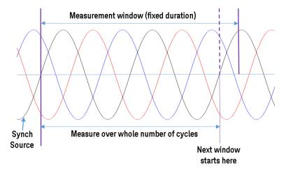
The sync source determines the measurement period. The other signals will be measured over an integer number of cycles if their frequencies match the sync source. This is important for 3-phase measurements, as all three phases must be measured simultaneously to properly calculate total power. Furthermore, accurate efficiency analysis requires simultaneous measurement of input and output power.
