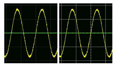
The grid lines correspond to the vertical and horizontal sensitivity settings shown at the top of the display. As shown below, the signal channels may have different vertical scales, but there is just one horizontal scale.
