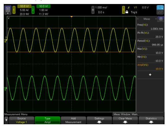
You can change the measurement for which cursors are displayed by touching the measurement in the list and choosing **Track With Cursors** or by selecting the measurement in the Cursors Menu.
