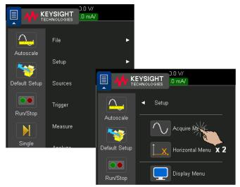
Touch left side controls to perform instrument operations.
