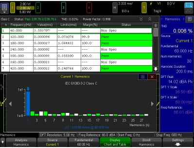
You can use the arrows on both sides of the bar chart to scroll through the chart, or you can press the **Scroll** softkey and turn the **Entry** knob. The table and chart always scroll together; if row 3 in the table is highlighted, the bar for harmonic 3 will turn blue, as shown below.
