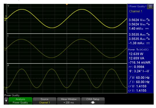
After selecting the Power Quality analysis, choose the Source (Channel 1 or Channel 2) to measure, and then configure CWA as usual. Note that you can also modify the CWA measurement window from either the main Power Quality menu or under the CWA Setup menu.
