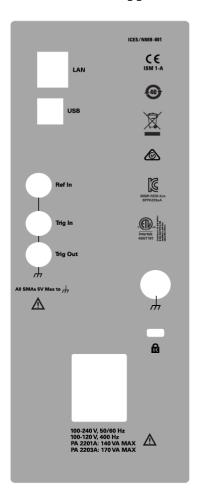
The outer shell of the Ref In, Trig In and Trig Out SMA connectors are connected directly to chassis. The maximum voltage that may be applied to the center conductor of these terminals with respect to the outer shell/chassis is 5 V.
