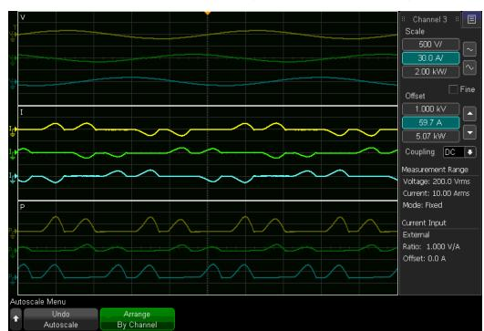
The image below shows the traces arranged by group. Note that all voltages are set to the same vertical scale, based on the largest voltage. This scaling principle also applies to current and power, and it enables you to quickly detect imbalances across channels. If a signal is relatively small, you always have the option to select the appropriate channel and adjust its scale individually.
