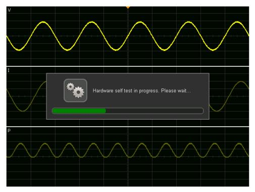
You should run Hardware Self Test after experiencing abnormal operation, for diagnostic information, or to verify proper operation after a repair.
