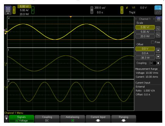
The ground level of the signal for each displayed signal is identified by the position of the icon at the far left side of the display.
