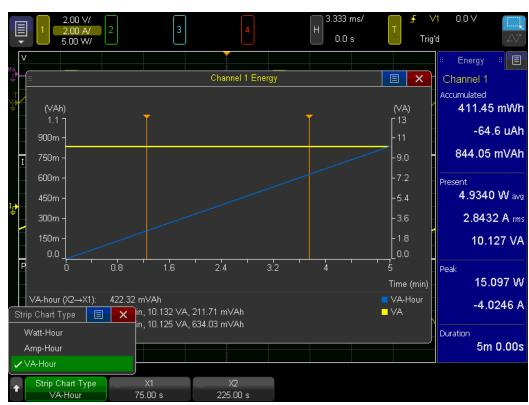
Also as mentioned above, you can change the cursor positions. The cursors in the previous image are 25% and 75% of the way through a 300-s analysis. The image below shows the cursors spread out to capture the middle four minutes of the analysis.
