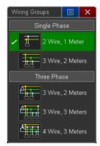
Note that the 3 Wire, 3 Meters and 4 Wire, 3 Meters choices are not available on the PA2201A.
