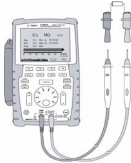
Figure 4 Connection for meter measurement
