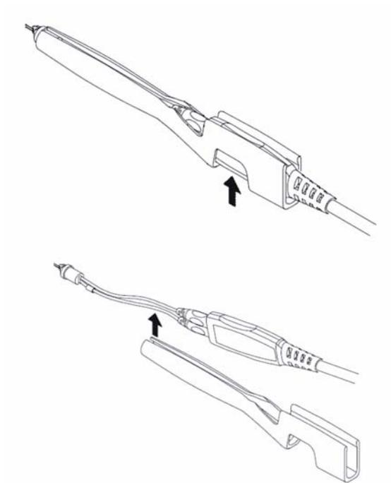
**Figure 1-6** Steps to remove the browser from the ergonomic handle
