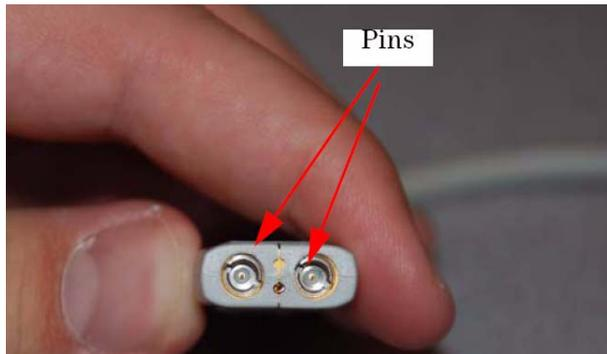
**Figure 1-3** Straight pins in an amplifier
